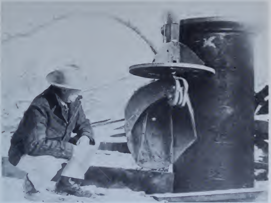
Figure 38.—“Core shovel” used to secure representative aggregate samples from cased test holes that cannot be dewatered. PX-D-32043.
